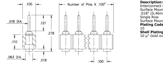
Interconnect Header Surface Mount Pin Header .018" (0,46mm) Pin Head Surface Mount **Plating Code:** Shell Plating: 10 µ" Gold over 100 µ" Nickel
