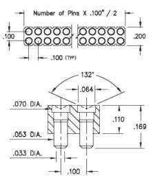
Description: Interconnect Target Connector Spring-Loaded Header Vertical Mount SMT Target with Concave Face Double Row Surface Mount Plating Code: 10
