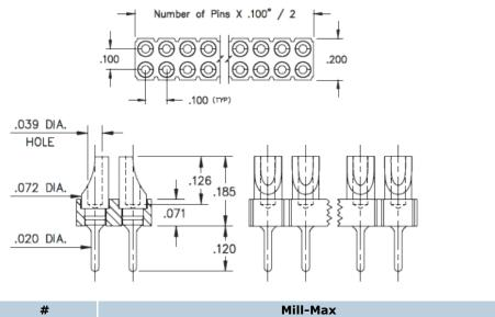
**Description:** Interconnect Header Solder Tail Pin Header SolderCup Head Double Row Through Hole Plating Code: 10 Shell Plating: 10  $\mu$ " Gold over 100  $\mu$ " Nickel
