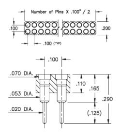
**Description:** Interconnect Target Connector Spring-Loaded Header Vertical Mount Through Hole Target Double Row Through Hole Plating Code: 10 Shell Plating: 10 µ" Gold over 100 µ" Nickel
