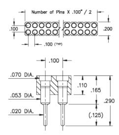
**Description:** Interconnect Flat Face Target Connector Spring-Loaded Header Vertical Mount Through Hole Target Double Row Through Hole Plating Code: Shell Plating: 10 μ" Gold over 100 μ" Nickel Packaging:
