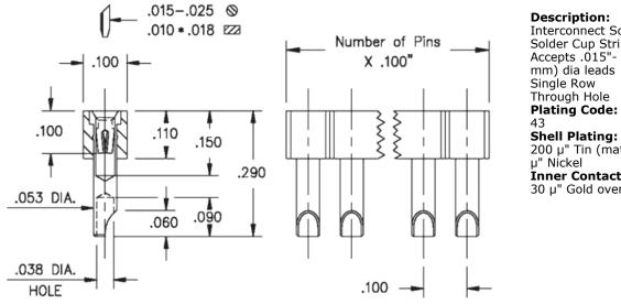
Interconnect Socket Solder Cup Strip Socket Accepts .015"- .025" (0,38 - 0,635 mm) dia leads Through Hole
