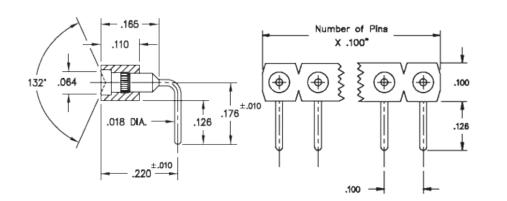
Description: Interconnect Target Connector Spring-Loaded Header Right Angle Mount Target with Concave Face Single Row Through Hole Plating Code: 10
