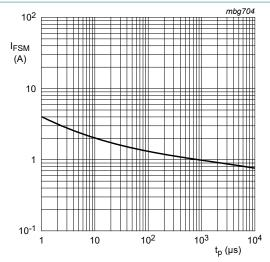
Based on square wave currents.  $T_{i(init)} = 25 \, ^{\circ}C$
