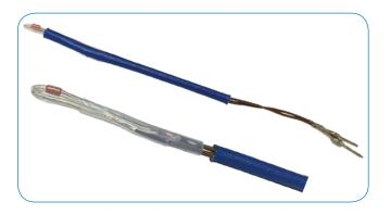
The A-1737 Motor Coil Temperature Sensor provides critical temperature feedback of an electric motor's operating condition. Used by either interlacing into the stator coil, or tied to the neutral bus bar on the motor circuit, it provides a temperature feedback to indicate motor load or stall conditions.
