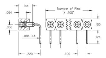
**Description:** Interconnect Socket Right Angle Socket Accepts .015" - .025" (0,38 - 0,635 mm) dia leads Single Row Through Hole **Plating Code:** Shell Plating: 10 μ" Gold over 100 μ" Nickel Inner Contact Plating: 10  $\mu$ " Gold over 50  $\mu$ " Nickel
