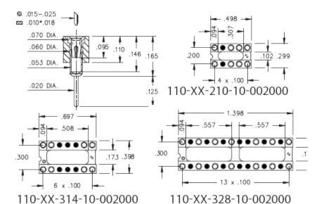
**Description:** DIP Dual In Line Socket Selectively Loaded Socket for Dual In Line Relays Open Frame Through Hole Plating Code: 13 Shell Plating: 10 μ" Gold over 100 μ" Nickel
