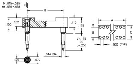
**Description:** DIP Dual In Line Socket Solderless Press-Fit Standard Tail Open Frame Through Hole Plating Code: Shell Plating: 10 μ" Gold over 100 μ" Nickel Inner Contact Plating: 30 μ" Gold over 50 μ" Nickel
