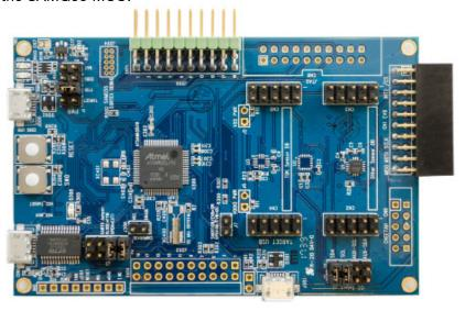
The development kit comes with evaluation software including MotionLink, a GUI based development tool and embedded motion drivers for both IAM-20680 and IAM-20680HP.
