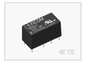
Contact Voltage Rating: 220 VDC Signal Relay Coil Power Rating (DC): 550 mW Isolation (HF Parameter): -20.7dB @ 900MHz, -39dB @ 100MHz Insertion Loss (HF Parameter): -.02dB @ 100MHz, -.27dB @ 900MHz
