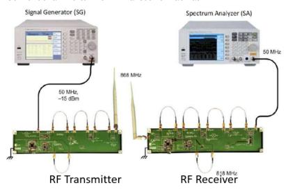
This lab setup can flexibly be configured with DAQ905A RF multiplexer as web-enabled remote RF lab task.
