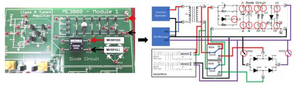
Multiples jumpers / test points / switches can be replaced with DAQ solution.
