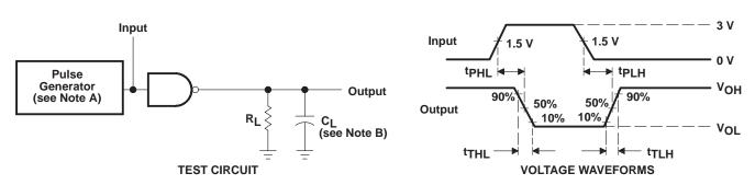
NOTES: A. The pulse generator has the following characteristics:  $t_W$  = 0.5  $\mu$ s, PRR  $\leq$  1 MHz,  $Z_O$  = 50  $\Omega$ .
