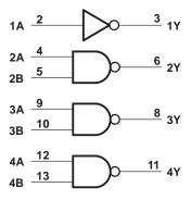
Positive logic  $Y = \overline{A} (driver 1)$  $Y = \overline{AB} \text{ or } \overline{A} + \overline{B} (drivers 2 \text{ thru 4})$
