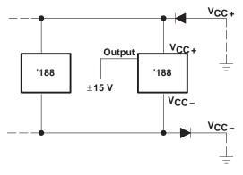
Diodes placed in series with the V<sub>CC+</sub> and V<sub>CC-</sub> leads protect the SN55188/SN75188 in the fault condition in which the device outputs are shorted to  $\pm 15$  V, and the power supplies are at low voltage and provide low-impedance paths to ground.
