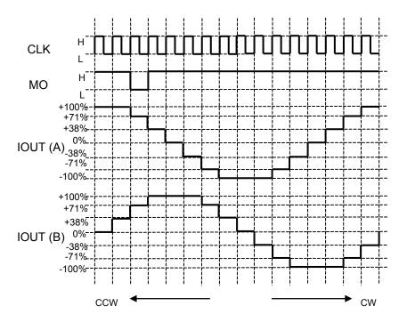
MO output shown in the timing chart is under the condition the MO pin is pulled up. Timing charts may be simplified for explanatory purpose.
