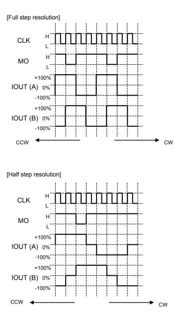
MO output shown in the timing chart is under the condition the MO pin is pulled up. Timing charts may be simplified for explanatory purpose.
