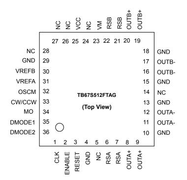
\*: Please mount the four-corner pads of the QFN package and the exposed pad to the GND area of the PCB.
