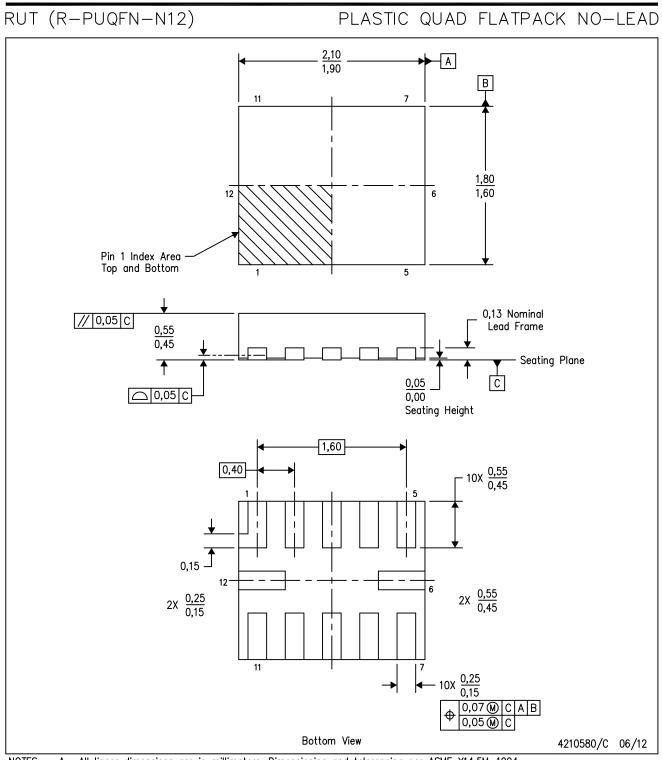
NOTES: All linear dimensions are in millimeters. Dimensioning and tolerancing per ASME Y14.5M-1994. Α.
