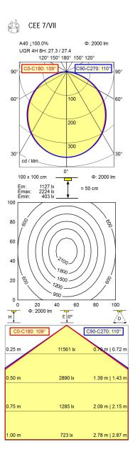
light sourceLEDwork equipmentelectronic transformerconnected load100-240 V, 50/60 Hz; secondary 24 V, DCpower consumptionenv. 30 W
