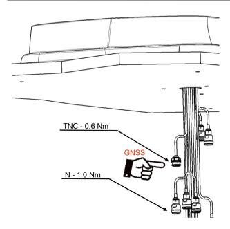
Connect the cables. Hold the pigtail connectors during cable attachment. Avoid all tension, torsion and bending forces.
