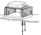
Use parts of the packaging to easily position the antenna above the cable breakthrough as indicated on the picture.
