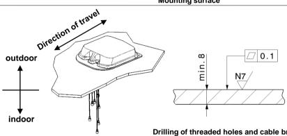
The mounting surface shall be planar and stable. The material of the mounting surface shall be steel or aluminium.
