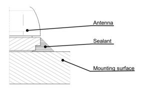
It is optional to seal the perimeter of the antenna with sealant
