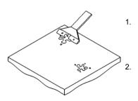
Clear the area where the bracket is welded from paint, corrosion or any anodized layer.
