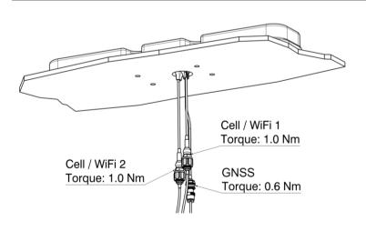
Connect the cables. Apply the indicated torque according to the connector.
