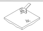
Clear the area where the antenna is mounted from paint, corrosion, anodized layer, dust, cutting chip, burrs, oil and fat.
