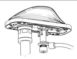
When mounting the antenna onto a bracket, the cable entry has to be protected against environmental impact. If the mounting surface doesn't fulfill the requirements mentioned above, the antenna has to be grounded using a separate grounding cable.
