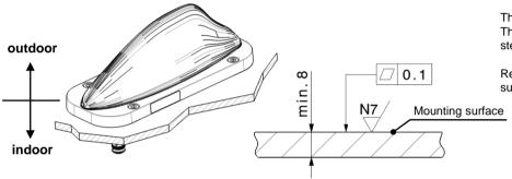
The mounting surface shall be planar and stable. The material of the mounting surface shall be steel or aluminium
