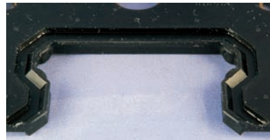
Lip has not been fractured
