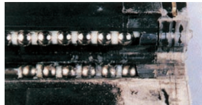
No. 1 Traveled 100 km (double-seal configuration)
