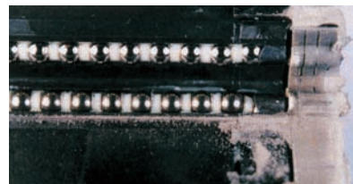
No foreign matter entering the raceway observed
