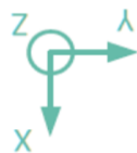
Figure 23: Field convention (Top view of the package with pin 1 at the bottom left)
