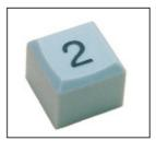
L 12mm, W 12mm, H 10mm CS-12 Designed to fit 3.3mm shaft of push button switches.
