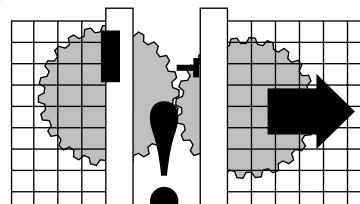
(a) Check the machine is isolated and stopped whenever the interlocked guard door is open.
