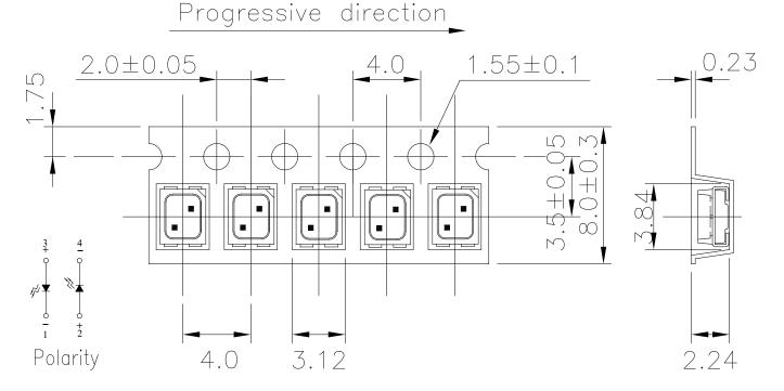
**Note:** The tolerance unless mentioned is  $\pm 0.1$ mm.
