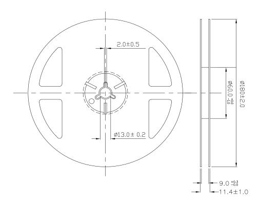
**Note:** The tolerance unless mentioned is  $\pm 0.1$ mm.
