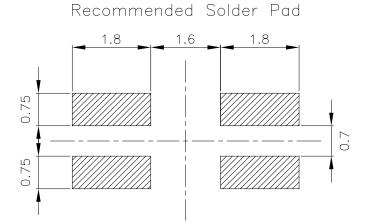
**Note:** The tolerance unless mentioned is  $\pm 0.1$ mm.
