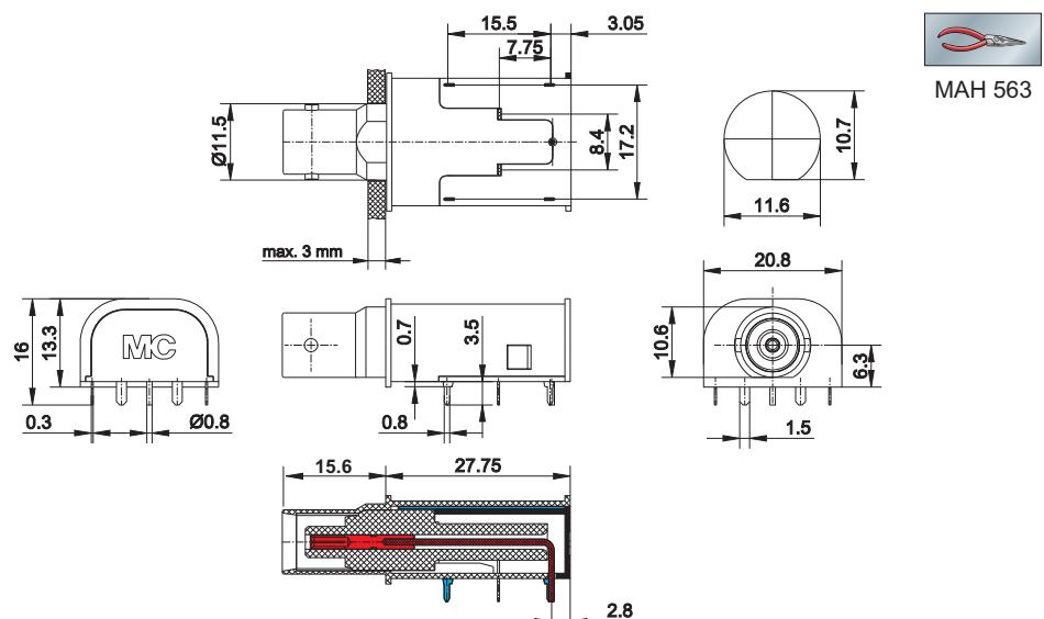
Touch-protected BNC angled socket for mounting on printed-circuit boards, touch-protected according to IEC / EN 61010-1. The socket is directly soldered onto printed-circuit boards. The right-angled configuration minimises the force transmitted to the printed-circuit board through the plugged-in test lead.
