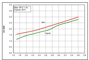
**FIGURE 36-20:** IDD, HFINTOSC Mode, Fosc = 32 MHz (PIC16LF18326/46 only)
