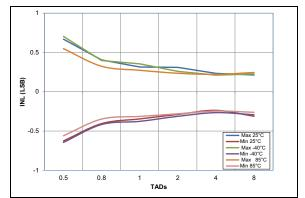
FIGURE 36-58: ADC 10-Bit Mode, Single-Ended INL, VDD = 3.0V, VREF = 3.0V (All devices)
