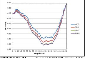
**FIGURE 36-74:** Typical DAC INL Error, VDD = 5.0V, VREF = External 5V (PIC16F18326/46 only)
