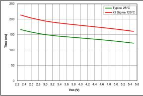
**FIGURE 36-91:** Comparator Response Time Falling Edge (PIC16F18326/46 only)
