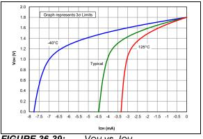
FIGURE 36-39: VOH vs. IOH Overtemperature, VDD = 1.8V (PIC16LF18326/46 only)
