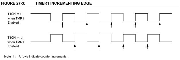
2: In Counter mode, a falling edge must be registered by the counter prior to the first incrementing rising edge of the clock.
