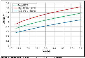
FIGURE 36-103: Input Level TTL
