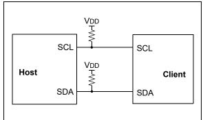
On the last byte of data communicated, the host device may end the transmission by sending a Stop <u>bit</u>. If the host device is in <u>Receive</u> mode, it sends a <u>NACK</u> in place of the last <del>ACK</del> bit. A Stop bit is indicated by a low-to-high transition of the SDA line while the SCL line is held high.
