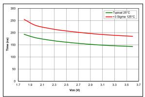
FIGURE 36-90: Comparator Response Time Falling Edge (PIC16LF18326/46 only)
