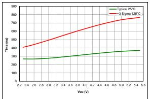
FIGURE 36-93: Comparator Response Time Rising Edge (PIC16F18326/46 only)
