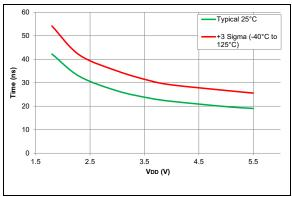
FIGURE 36-105: Fall Time, Slew Rate Control Enabled
