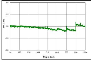
**FIGURE 36-55:** ADC 10-Bit Mode, Single-Ended INL, VDD = 3.0V, VREF = 3.0V, TAD =  $4 \mu s$ , 25C (All devices)
