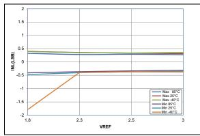
**FIGURE 36-60:** ADC 10-Bit Mode, Single-Ended INL, VDD = 3.0V, TAD =  $1 \mu$ s (All devices)
