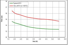
FIGURE 36-113: Wake From Sleep, VREGPM = 0, HFINTOSC = 4 MHz (PIC16F18326/46 only)
