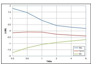
**FIGURE 36-68:** ADC 10-Bit Mode, Single-Ended Offset Error, VDD = 3.0V, VREF = 3.0V, -40°C to 85°C(All devices)
