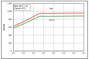
FIGURE 36-27: IDD, HFINTOSC Doze Mode, Fosc = 16 MHz (PIC16F18326/46 only)
