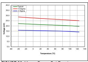
FIGURE 36-44: Brown-Out Reset Hysteresis, Trip Point (BORV = 1) (PIC16LF18326/46 only)
