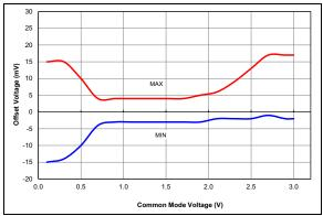
**FIGURE 36-81:** Comparator Offset, Normal Power Mode (CxSP = 1), VDD = 3.0V, Typical Measured Values at 25°C
