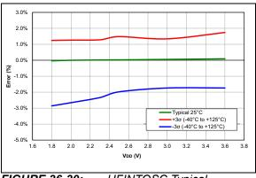
FIGURE 36-30: HFINTOSC Typical Frequency Error (PIC16LF18326/46 only)
