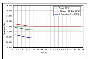
FIGURE 36-29: LFINTOSC Frequency (PIC16F18326/46 only)
