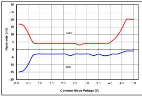
**FIGURE 36-84:** Comparator Offset, Normal Power Mode (CxSP = 1), VDD = 5.0V, Typical Measured Values at 25°C
