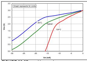
FIGURE 36-37: VOH vs. IOH Overtemperature, VDD = 3.0V (All devices)
