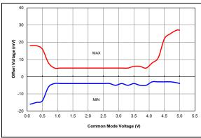
**FIGURE 36-85:** Comparator Offset, Normal Power Mode (CxSP = 1), VDD = 5.5V, Typical Measured Values from -40°C to 125°C
