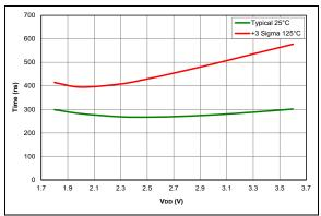
**FIGURE 36-92:** Comparator Response Time Rising Edge (PIC16LF18326/46 only)
