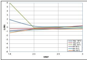
**FIGURE 36-61:** ADC 10-Bit Mode, Single-Ended Gain Error, VDD = 3.0V, TAD = 1 μs (All devices)
