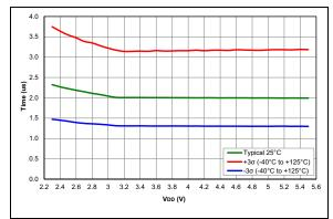
FIGURE 36-70: ADC RC Oscillator Period (PIC16F18326/46 only)
