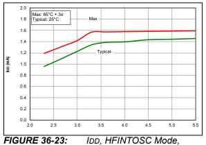
FIGURE 36-23: IDD, HFINTOSC Mode Fosc = 16 MHz (PIC16F18326/46 only)
