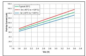
FIGURE 36-34: Weak Pull-Up Current (PIC16LF18326/46 only)
