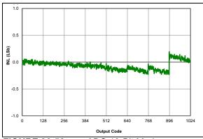
**FIGURE 36-56:** ADC 10-Bit Mode, Single-Ended INL, VDD = 3.0V, VREF = 3.0V, TAD =  $8 \mu s$ , 25C (All devices)
