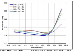
FIGURE 36-78: Absolute Value of DAC DNL Error, VDD = 5.0V, VDD = 5.0V, VREF = VDD (PIC16F18326/46 only)
