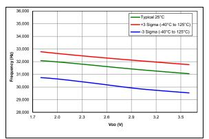
FIGURE 36-28: LFINTOSC Frequency (PIC16LF18326/46 only)
