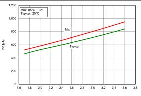
FIGURE 36-24: IDD, HFINTOSC Idle Mode, Fosc = 16 MHz (PIC16LF18326/46 only)
