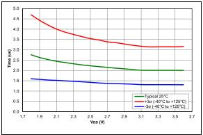
FIGURE 36-69: ADC RC Oscillator Period (PIC16LF18326/46 only)
