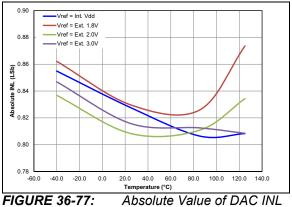
FIGURE 36-77: Absolute Value of DAC INL Error, VDD = 3.0V, VREF = VDD (All devices)
