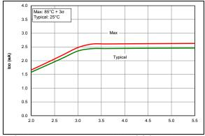
**FIGURE 36-21:** IDD, HFINTOSC Mode, Fosc = 32 MHz (PIC16F18326/46 only)
