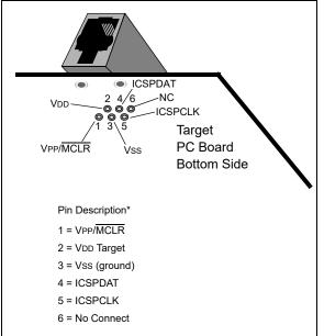
Another connector often found in use with the PICkit<sup>™</sup> programmers is a standard 6-pin header with 0.1 inch spacing. Refer to Figure 33-2.
