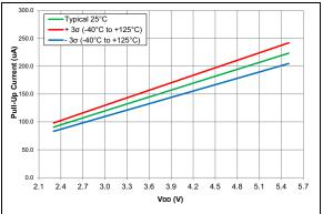
FIGURE 36-33: Weak Pull-Up Current (PIC16F18326/46 only)
