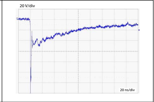
Figure 8. ESD response to ISO 10605, C = 150 pF, R = 330 Ω (-8 kV contact)
