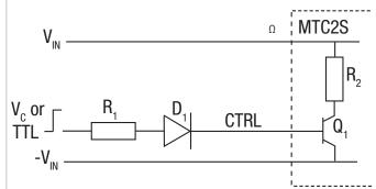
$D_{_1}$  (e.g. 1N4001) is necessary for correct operation of the MTC2 when the control signal is LOW. The recommended drive current  $I_{_B}$  to shut down the MTC2 is 6mA to 15mA. The value of R, can be derived as follows:
