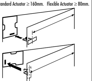
(c) Actuator must enter switch aperture centrally in line and not strike switch body. **STOP**
