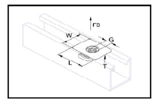
Material: Channel nut (verz.) from S460MC, with zinc plated; or Channel nut (DT) from S460MC, with Delta Tone; or Channel nut (A4) from 1.4404 (Sainless Steel 316) Plastic component from Polyamid (PA6)
