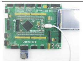
·Message/info will be displayed on the LCD and SD card hard disk will be founded in the PC.
