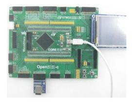
Host mode: Connect the Core board and the USB Flash Drive by the USB OTG cable. As shown in the figure below:
