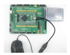
Part 1: When running DEVICE DEMO, you should find the SD card appears as a USB Flash Drive on the PC.
