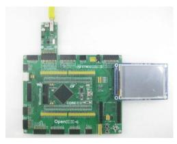
·Part 2: Connect a USB mouse or keyboard to the onboard FS USB interface through a USB OTG cable, short 3 jumpers PC2-FLG, PC1-PWROUT, PA9-VBUS. As shown in the figure below:
