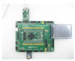
Message will be displayed on the LCD; SD card hard disk will be founded in the PC.
