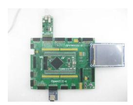
·Part 2: Connect the core board (FS USB interface) and PC by USB cable; Short the 3 jumpers PC2-FLG, PC1-PWROUT, PA9-VBUS. As shown in the figure below:
