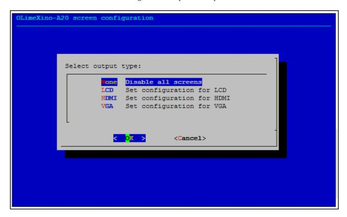
Choose the resolution and the interface (LCD, HDMI or VGA).
