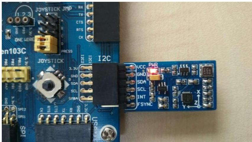
Figure 1: Connection between 10 DOF IMU Sensor (B) module and STM32
