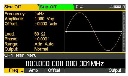
With the edit cursor positioned at the required digit the knob may be rotated left or right to decrement or increment the digit. As the value passes between 9 and 0 the digits to the left will also change. In this way it is possible to set any legal value for the parameter.
