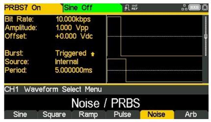
Notice that Triggered still shows in the Burst field of the Parameters Box and the BURST key still glows, indicating that burst is still active. To return to the Burst menu to edit the burst parameters press the BURST key again. To turn off burst press the On/Off soft-key in the burst menu.
