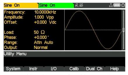
Press **Instr** soft-key and then press **FrCntr** soft-key to access the counter capabilities of the instrument.
