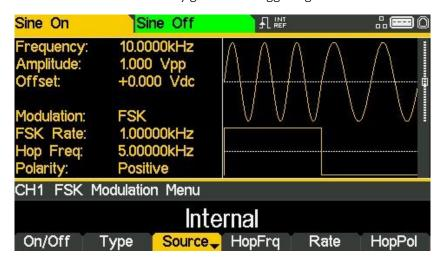
External will use the signal present at the TRIG / COUNT (DC) IN connector and the Rate parameter will no longer be editable. The Graph Box will show a switching carrier and a square-wave as the modulating waveform irrespective of the source of the switching signal.
