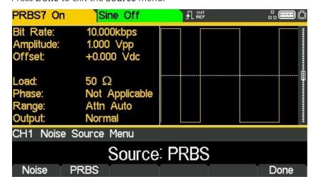
Press the Type soft-key to set PRBS type. The soft-keys PN7, PN9, PN11, PN15, PN20, PN23, PN29 and PN31 set the number of bits used to generate the PRBS.
