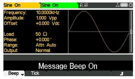
Tick refers to the sound made when the front panel keys are pressed, when activated the screen will read **Key Tick On** and each key press will make a short sound. These sounds are suppressed with **Key Tick Off**.
