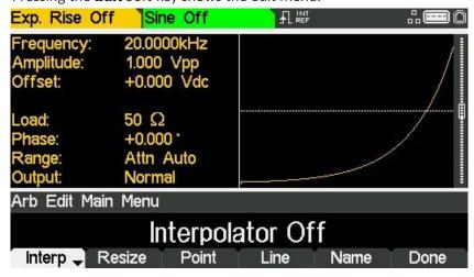
While editing an arbitrary waveform, if the same arbitrary waveform is also currently selected to be the output, then the changes made to the arbitrary waveform can be observed in real time. The waveform will be available at the MAIN OUT connector of the selected channel for display on an oscilloscope. There will also be a representation shown in the Graph Box.
