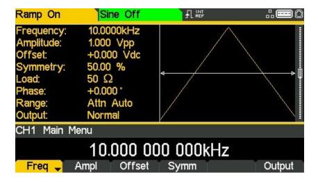
The orange channel 1 indicator tab shows that the waveform is set to ramp and the Graph Box has changed to show the ramp waveform.
