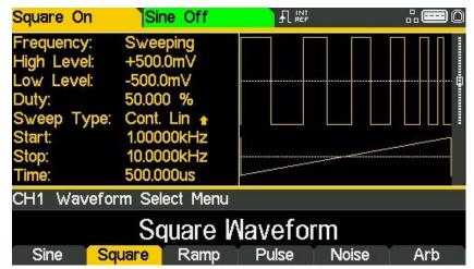
Notice that **Sweeping** still shows in the **Frequency** field of the Parameters Box and the SWEEP key still glows, indicating that sweep is still active.
