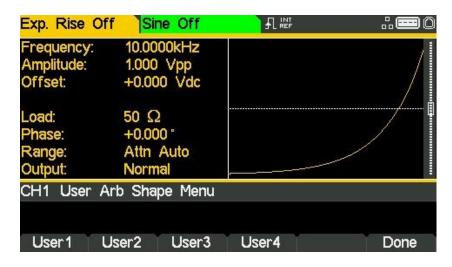
The four soft-keys **User1** through **User4** allows direct access to the user-defined arbitrary waveforms in the instrument. To select an arbitrary waveform, press the appropriate soft-key. Press the **Done** soft-key to return to the top-level **Arb** menu.
