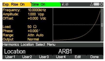
The name of the arb selected for storing the harmonic waveform is shown in the Edit Box. To select an arbitrary waveform location for storing the harmonic waveform press the appropriate soft-key.
