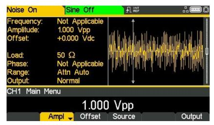
It is possible to edit these parameters in terms of high level and low level by pressing the Ampl key.
