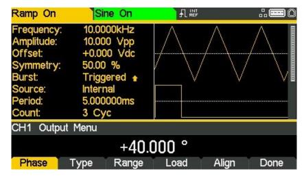
The carrier waveform in the Graph Box will show a representation of the carrier start phase as the phase is edited.
