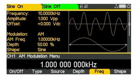
The Parameters Box on the right-hand side now shows AM in the Modulation field and the current modulation parameters of AM Freq, Depth and Shape. The Graph Box shows the modulating waveform below a representation of the modulated carrier waveform.
