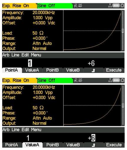
The **PointB** and **ValueB** soft-keys are used to set the second point. The line is drawn in the actual waveform by pressing the **Execute** soft-key after which the instrument will return to the top-level edit menu.
