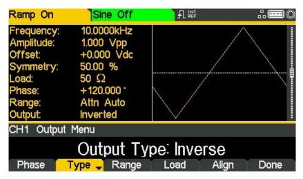
**Inverse** will invert the carrier waveform at the MAIN OUT connector. The output is set to **Inverted** in the parameters box and the carrier waveform in the Graph Box will be inverted.
