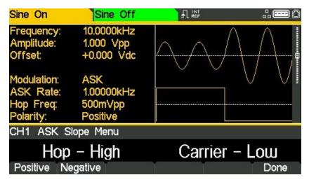
Setting **Negative** will cause ASK to generate the hop amplitude while the switching signal is low and the carrier amplitude while the switching signal is high.
