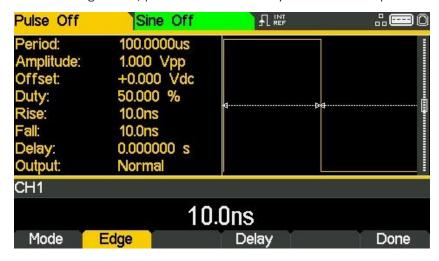
The edge time represents the time between the 10% and 90% points on the pulse edges. Rise time and fall time can be coupled or adjusted independently.
