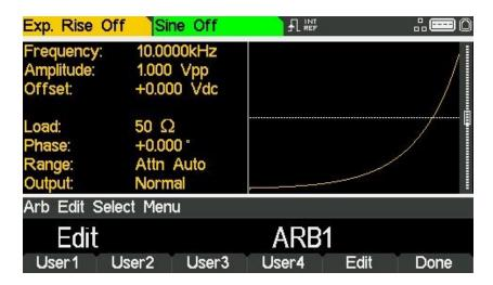
The instrument is capable of performing simple editing of stored arbitrary waveforms. For more complex editing and creation of waveforms see the Waveform Manager Plus V4.13 Windows application, available on the website: <a href="https://www.aimtti.com">www.aimtti.com</a>
