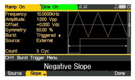
The trigger waveform in the Graph Box changes to show the edge in use.
