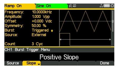
Repeated presses of the Slope soft-key will select between Positive Slope and Negative Slope.
