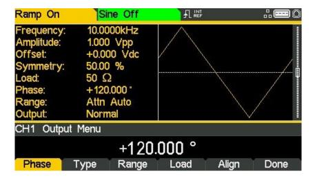
The setting may be used to determine the phase difference between the two channels or between channel 1 waveform and its carrier sync. The channels may be phase aligned by pressing the **Align** soft-key. The Phase parameter is also used to set Burst Phase.
