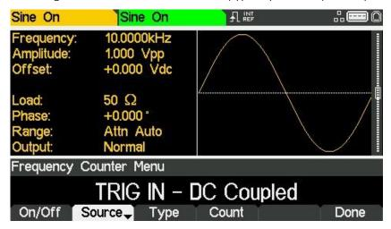
The REF / COUNT (AC) IN socket is AC coupled. Select this input to count signals from 3Hz to >125MHz (typically 150MHz). The input sensitivity is 100mV.
