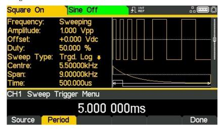
When the source is external trigger, the **Period** soft-key is replaced by **Slope** soft-key.
