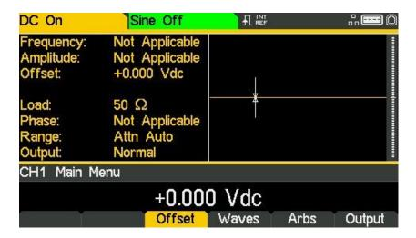
The orange channel 1 status line shows DC in the Waveform field, the Graph Box shows a DC waveform with DC offset arrows and the Edit Box contains the DC voltage menu.
