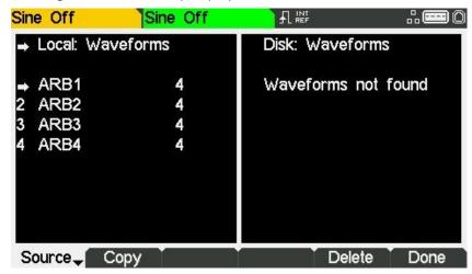
There are four local arbitrary waveform stores numbered 1 to 4. The number is shown next to the file name in the Local: Box. Initially the files are all set to the default four-point squarewave. The file names are set as ARB1 to ARB4 by default but they may be changed as they are used.
