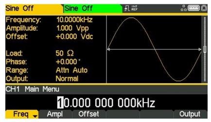
Layout 2: Shows the parameters for both channels simultaneously.
