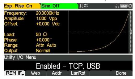
The default is for all available interfaces to be enabled as shown. The REM IF soft-key may be used to select the interfaces required. Pressing the REM IF key will cycle round the possibilities, in this case:
