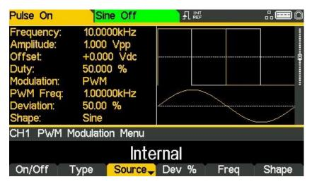
External will use the signal present at the MOD IN connector and the Freq and Shape parameters will no longer be editable. The Graph Box will always show a sinewave as the modulating waveform if the source is set to external.
