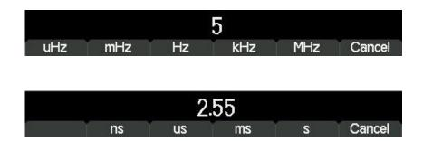
During the numeric data entry, a decimal point and, if appropriate, a sign may be entered. The +/- key is used to alternately change the sign between + and –. The left cursor key may be used to erase the last digit entered. The entry may be cancelled by pressing the Cancel key
