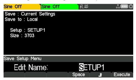
The name offered will be the same as the name in the selected set-up store when the Save soft-key was pressed. The Edit Box shows the name of the file that will be saved and the soft-key labels. The KNOB and cursor keys allow the name to be edited.
