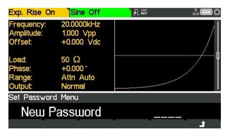
Enter a 4—digit password from the keyboard; the Edit Box will show the message Confirm. Reenter the password and the message new password stored will pop up for two seconds before returning to the top-level calibration menu.
