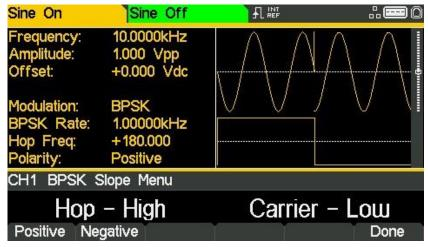
Setting **Negative** will cause BPSK to generate the hop phase while the switching signal is low and the carrier phase while the switching signal is high.
