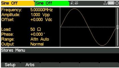
Pressing the Setup soft-key displays the setup sub-menu.
