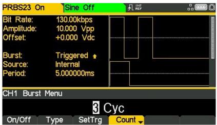
The carrier waveform in the Graph Box will show a representation of the burst as the count is edited.
