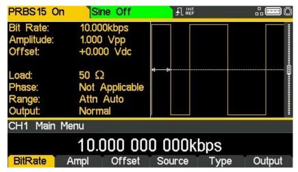
Use the Ampl and Offset soft-keys to set these parameters as for any other carrier wave.
