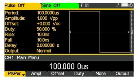
Amplitude and dc offset are adjusted in the same way as for sine waves and they may also be set in terms of high level and low level.
