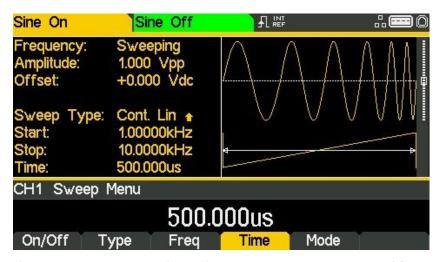
The Parameters Box now shows the current sweep parameters of **Sweep time**, **Start**, **Stop** and **Time**, and **Sweeping** is shown in the **Frequency** field. The Graph Box shows the sweep waveform type below a representation of the swept carrier waveform. The Edit Box contains the selected parameter, in this case sweep time.
