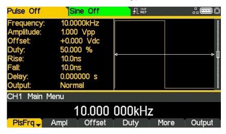
The PlsFrq soft-key allows setting of the pulse frequency. Pressing the key while it is highlighted will change it to PlsPer and the pulse period may be entered. The pulse generator uses its own value for pulse frequency/pulse period. Changing it will not affect the frequency/period value of the other carrier waveforms.
