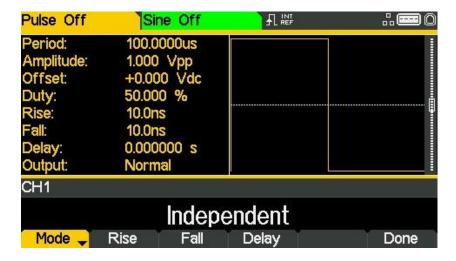
The parameters box will show Rise and Fall at all times, the values will change depending on whether coupled or independent mode has been selected.
