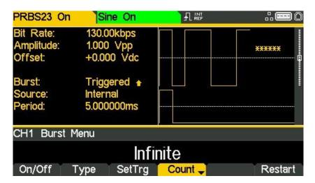
When the number of cycles is infinite, the trigger starts the waveform. Press the **Restart** soft-key to stop the waveform and wait for a trigger to re-start the waveform.
