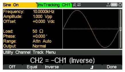
When either tracking option is enabled the waveforms will remain aligned at a phase of 0°.
