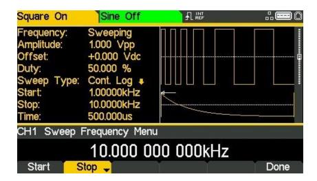
The frequency parameter will appear in the Edit Box and the sweep waveform type in the Graph Box will show that start or stop frequency is being edited.
