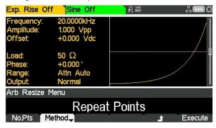
When a waveform is increased in size new points are added between existing points. The way that the values of these new points are calculated depends on the resize method setting, The **Repeat Points** method adds points of the same value as the original point in the waveform. The **Interpolate** method draws a straight line between the existing points.
