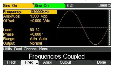
When entering frequency coupling modes, the instrument will automatically phase align the channels. The phases may become misaligned by subsequent parameter changes. To realign the phase at any time, press the **Align** soft-key from the carrier- output menu.
