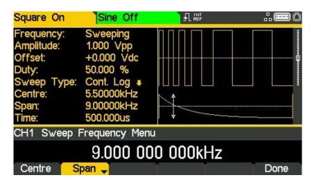
With centre/span mode selected the Edit Box shows the parameter, the Parameters Box shows Centre and Span in place of Start and Stop and the Graph Box changes to show the parameter which is being edited.
