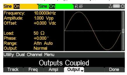
It is possible to set any combination of Frequency, Amplitude and Output coupling.
