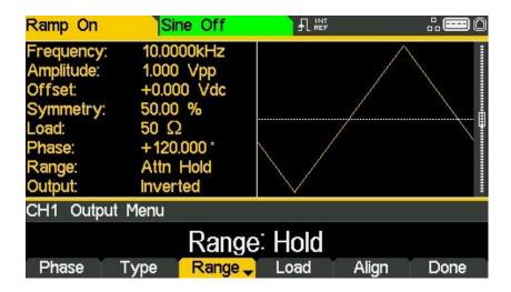
With range set to **Hold** a fixed attenuator setting is used for all amplitude settings. The **Range** field in the Parameters Box will show **Attn Hold** while range is held.
