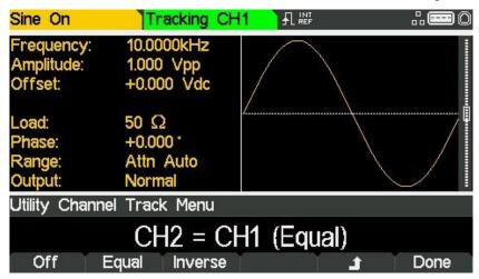
Tracking may be inverted by pressing the **Inverse** soft-key to produce a differential pair of signals.
