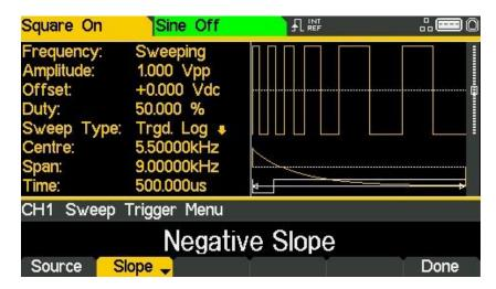
When the source is manual trigger, there are no additional parameters to be set. Press the TRIGGER key to send a manual trigger. Press the **Done** soft-key to return to the top-level sweep menu.
