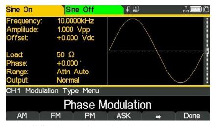
Press On/Off soft-key to apply the selected modulation.
