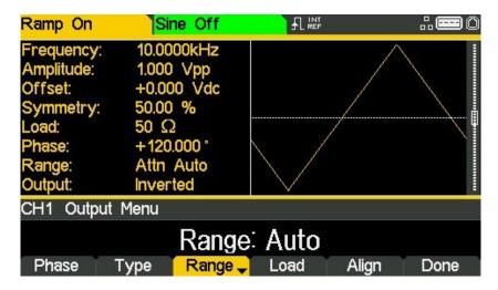
Selecting Hold mode disables auto-ranging; the attenuator setting is fixed for the unit's maximum amplitude. This can be useful in eliminating momentary disruptions in the output waveform in Auto mode caused by the switching of the attenuators while changing the amplitude. However, waveform quality will start to deteriorate at lower amplitudes.
