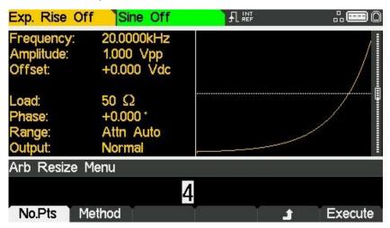
The **No.Pts** soft-key allows the new size to be specified. Press the **Execute** soft-key to resize the waveform and return to the top-level edit menu. Pressing the soft-key will return without resizing.
