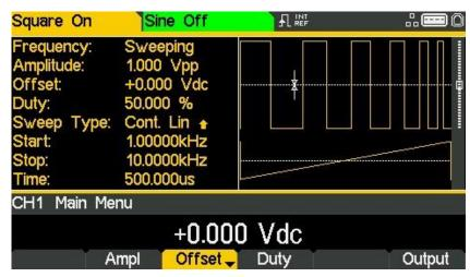
To return to the Sweep menu to edit the sweep parameters press the SWEEP key again. To turn off sweep press the On/Off soft-key in the sweep menu.
