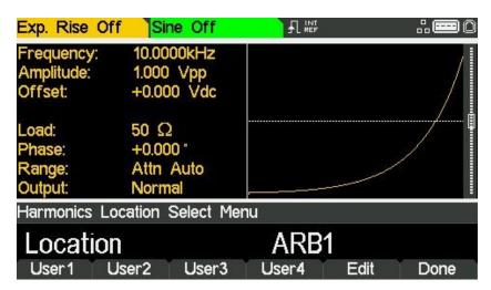
The instrument is capable of creating waveforms by the addition of sine wave harmonics. Up to 16 harmonics can be used, chosen from up to the 50<sup>th</sup> order. The amplitude and phase can be individually set for each harmonic. Harmonic waveforms can also be created or edited in the Waveform Manager Plus V4.13 Windows application supplied on the website: www.aimtti.com
