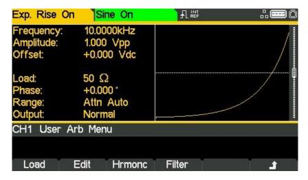
Pressing the Hrmonc soft-key opens the harmonic waveform sub-menu.
