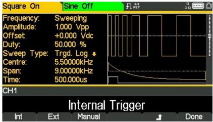
Pressing the **Period** soft-key allows the period of the internal trigger generator to be set. The Edit Box shows the current period and the Graph Box changes to show that the trigger period is being edited.
