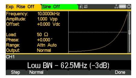
The instrument includes two filters to smooth transitions between points as arbitrary waveforms are generated. The Step filter has a nearly ideal step response, but with more roll-off in its frequency response than the Normal filter. The Normal filter has a wide, flat frequency response, but its step response exhibits overshoot and ringing.
