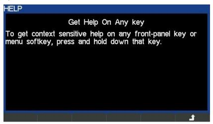
Below the topic heading is the topic text. If there is more text than will fit on the screen press the \$\infty\$ soft-key to scroll the text up one line.
