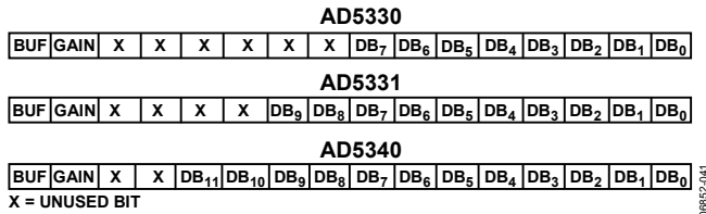
Figure 40. GAIN and BUF Data on a 16-Bit Bus
