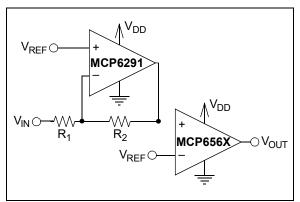
FIGURE 4-12: Precise Inverting Comparator.
