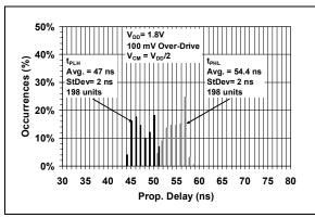
FIGURE 2-21: Low-to-High and High-to-Low Propagation Delays.
