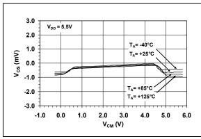
**FIGURE 2-9:** Input Offset Voltage vs. Common-Mode Input Voltage.
