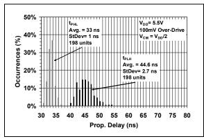
FIGURE 2-24: Low-to-High and High-to-Low Propagation Delays.
