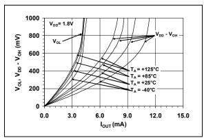
**FIGURE 2-20:** Output Headroom vs. Output Current.
