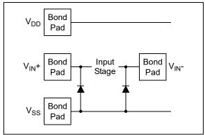
FIGURE 4-2: Simplified Analog Input ESD Structures.
