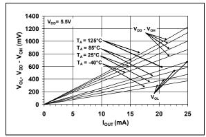
**FIGURE 2-23:** Output Headroom vs. Output Current.
