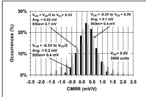
FIGURE 2-36: Common-Mode Rejection Ratio (CMRR).
