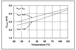
**FIGURE 2-10:** Input Hysteresis Voltage vs. Temperature.
