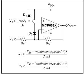
FIGURE 4-3: Protecting the Analog Inputs.
