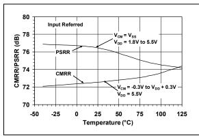
**FIGURE 2-33:** Common-Mode Rejection Ratio and Power Supply Rejection Ratio vs. Temperature.
