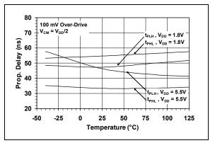
**FIGURE 2-28:** Propagation Delay vs. Temperature.
