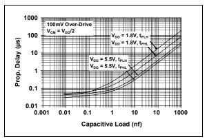
**FIGURE 2-31:** Propagation Delay vs. Capacitive Load.
