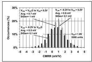
**FIGURE 2-35:** Common-Mode Rejection Ratio (CMRR).
