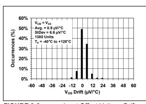
FIGURE 2-2: Input Offset Voltage Drift.
