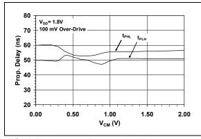
**FIGURE 2-27:** Propagation Delay vs. Common-Mode Input Voltage.
