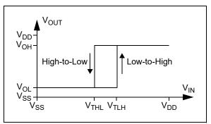
**FIGURE 4-5:** Hysteresis Diagram for the Noninverting Circuit.
