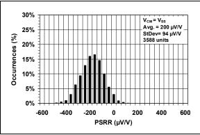
**FIGURE 2-34:** Power Supply Rejection Ratio (PSRR).
