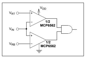
FIGURE 4-13: Windowed Comparator.
