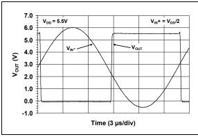
**FIGURE 2-3:** Input vs. Output Signal, No Phase Reversal.
