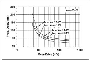
**FIGURE 2-29:** Propagation Delay vs. Input Overdrive.
