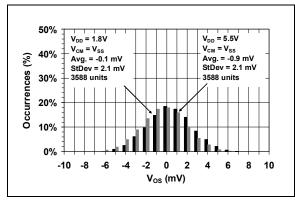
FIGURE 2-1: Input Offset Voltage.
