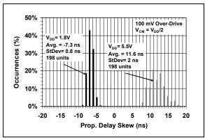
FIGURE 2-25: Propagation Delay Skew.
