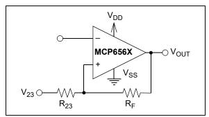
FIGURE 4-8: Thevenin Equivalent Circuit.
