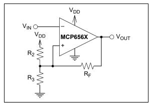
FIGURE 4-6: Inverting Circuit with Hysteresis.
