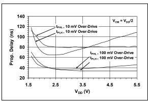
**FIGURE 2-26:** Propagation Delay vs. Supply Voltage.
