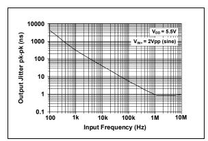
**FIGURE 2-37:** Output Jitter vs. Input Frequency.
