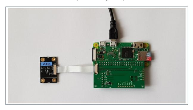
The TMF8x0x is shown when placing the Raspberry PI Zero W on the backside (see Figure 4)
