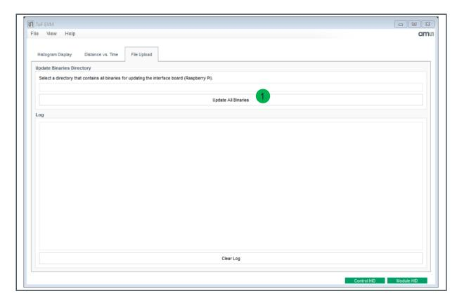
Press "Update All Binaries" – see 1 above – and select directory where the new firmware is located. Use "Select Folder" in the directory selection box to start the firmware upgrade. Power cycle the EVM once firmware upgrade is finished (see Figure 8).
