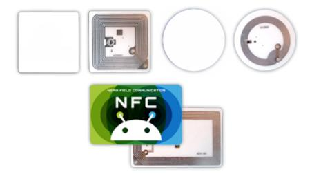
Type 1 tag is based on ISO/IEC 14443A standard and has 512 bytes of memory. Type 2 tag is based on ISO/IEC 14443A standard and has 192 bytes of memory. Type 4 is based on ISO / IEC 14443A 1-4 compliant and has 2K of memory.
