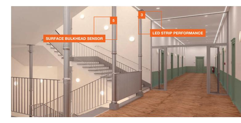
To minimize the risk of stumbling on stairs, the individual steps have to be in clear contrast to each other. Wide-beam luminaires projecting light down from the top landing provide short, soft shadows, making each step easy to see.
