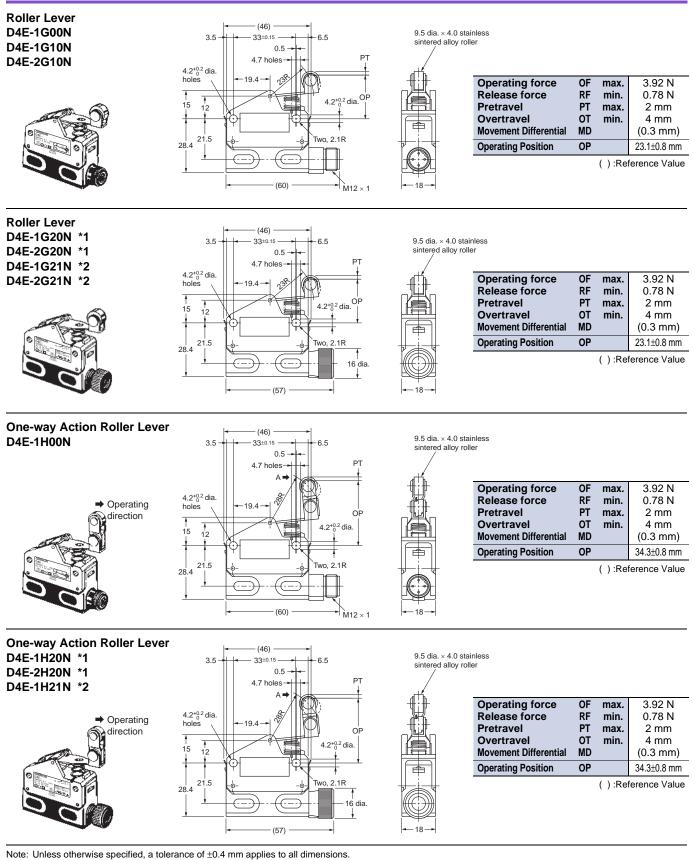
\*1. A 5.8-dia. to 7.6-dia. cable can be applied to the seal rubber for the lead wire outlet.
