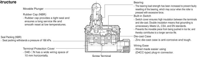
Screw terminal incorporates a M3 screw with a toothed washer.
