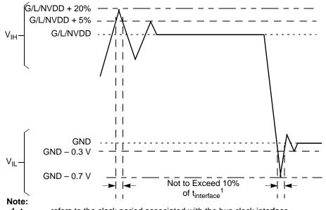
1.  $t_{\mbox{interface}}$  refers to the clock period associated with the bus clock interface.
