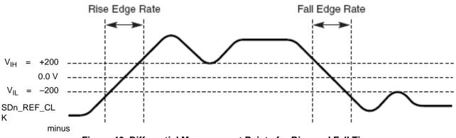
Figure 46. Differential Measurement Points for Rise and Fall Time
