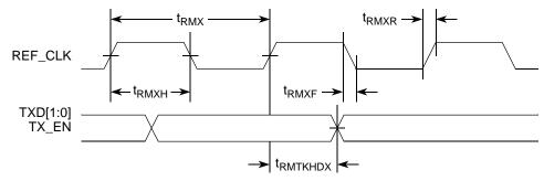
Figure 12. RMII Transmit AC Timing Diagram
