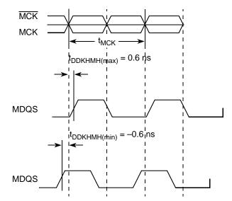
Figure 6. Timing Diagram for t<sub>DDKHMH</sub>
