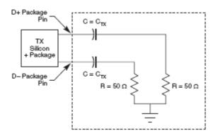
Figure 51. Compliance Test/Measurement Load
