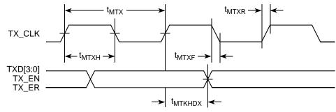
Figure 9. MII Transmit AC Timing Diagram
