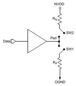
Figure 62. Driver Impedance Measurement
