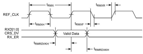
Figure 14. RMII Receive AC Timing Diagram
