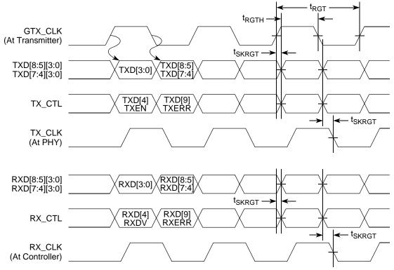
This figure shows the RGMII and RTBI AC timing and multiplexing diagrams.
