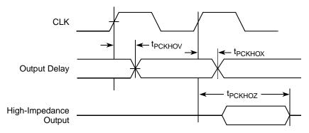
Figure 36. PCI Output AC Timing Measurement Condition
