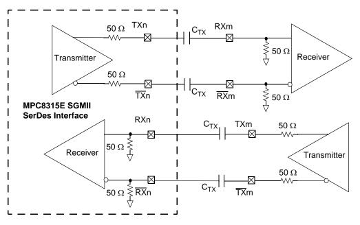
Figure 17. 4-Wire AC-Coupled SGMII Serial Link Connection Example
