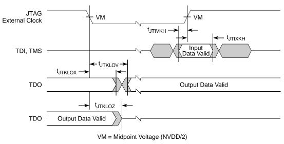
Figure 31. Test Access Port Timing Diagram
