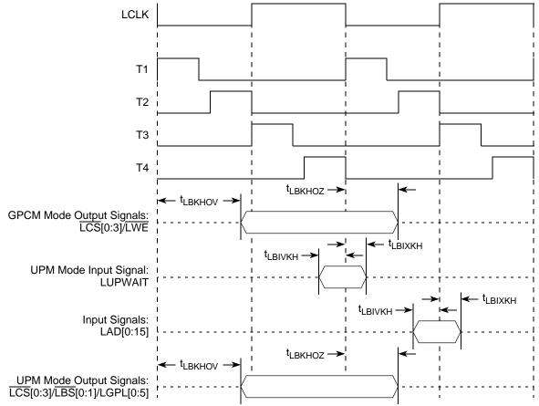
Figure 26. Local Bus Signals, GPCM/UPM Signals for LCRR[CLKDIV] = 4
