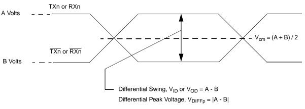
Differential Peak-Peak Voltage, VDIFFpp = 2\*VDIFFp (not shown)
