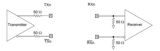
Figure 48. SerDes Transmitter and Receiver Reference Circuits
