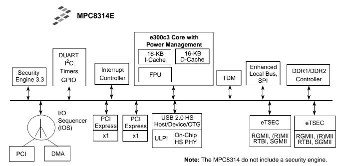
Figure 1. MPC8314E Block Diagram
