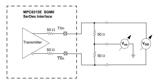
Figure 18. SGMII Transmitter DC Measurement Circuit
