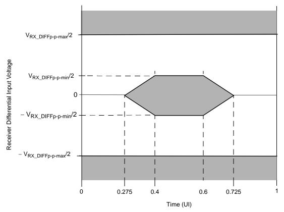
Figure 19. SGMII Receiver Input Compliance Mask
