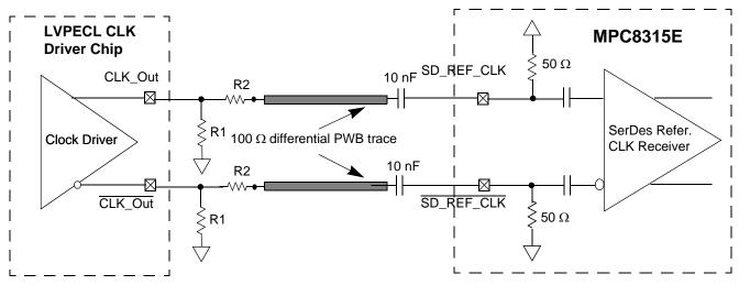
Figure 44. AC-Coupled Differential Connection with LVPECL Clock Driver (Reference Only)
