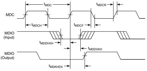
Figure 16. MII Management Interface Timing Diagram
