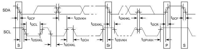
Figure 33. I<sup>2</sup>C Bus AC Timing Diagram
