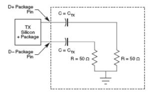
Figure 20. SGMII AC Test/Measurement Load
