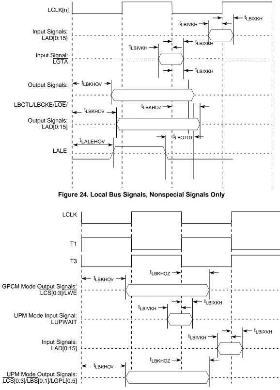
Figure 25. Local Bus Signals, GPCM/UPM Signals for LCRR[CLKDIV] = 2
