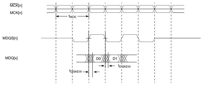
Figure 5. Timing Diagram for t<sub>DISKEW</sub>
