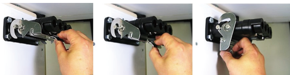
JK11 disengagement operation (Pinch the lock while pushing the lever down to disengage)
