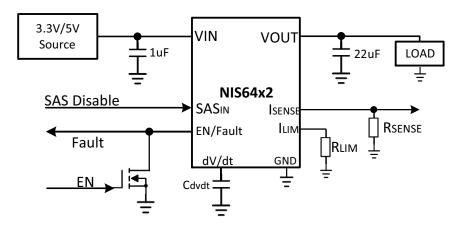
Figure 1. Typical Application Circuit
