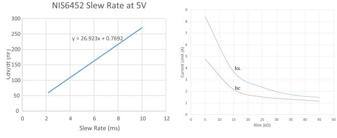
Figure 4. Slew Rate vs Cdvdt capacitance for 5V mode
