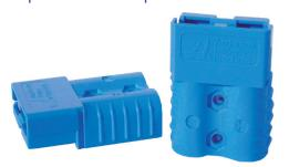
Like the other Multipole connectors, the SB\* 120 offers color-coded mechanically keyed housings. Keys can be used to identify and separate different circuits, or prevent users from accidentally cross mating different voltages. Wires sizes from 10 to 1 AWG (5.3 to 42.4 mm²) are held in the second smallest SB\* housing.
