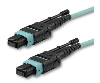
This MPO/MTP fiber optic cable houses 12 fibers and lets you interface between different networking devices of varying speeds. For example, you can set up a one-to-one connection between two 40Gbps switches or servers. Alternatively, you can connect a 40Gbps switch and break out the 40Gbps into six duplex 10Gbps LC connections on a patch panel or network cassette, which then fans out to individual 10Gbps devices.
