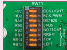
Figure 21-3: Enabled SW11.4 DIP switch
