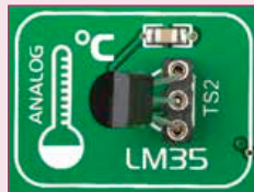
Figure 21-2: LM35 correctly placed in socket
