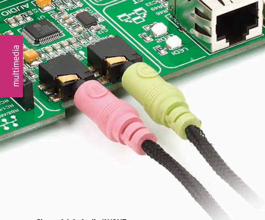
Figure 14-1: Audio IN/OUT connection schematic
