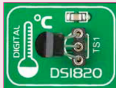
Figure 20-2: DS1820 correctly placed in socket
