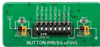
Figure 6-5: Button press level DIP switch (tri-state)
