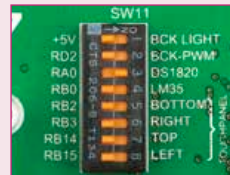
Figure 20-3: Enabled SW11.3 DIP switch
