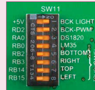
Figure 16-2: Turn on switches SW11.1 and SW11.2 to enable back- light and PWM signal from microcontroller.
