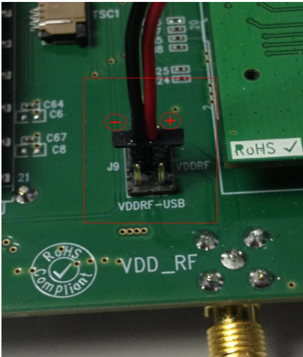
Figure 16 (Powering the ADF7023 Directly from Header J9)
