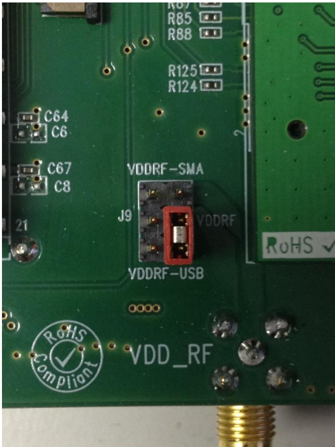
Figure 14 (Default Jumper configuration)
